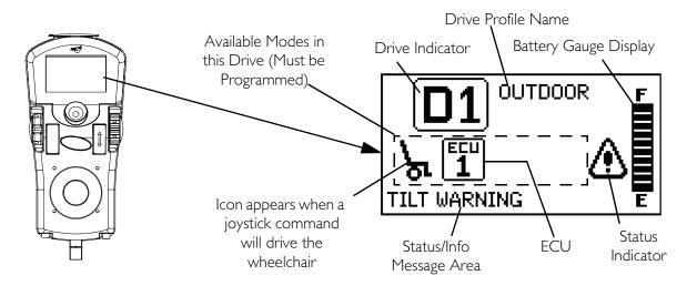
FIGURE 5.5 LCD Display Screens - Main Screen
